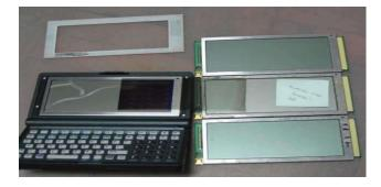
In the photo above, the HPLX unit on the left has already been stripped off its spoilt polarizer sheet. The polarizer sheet from the donor screen unit [right middle] appeared very dark when placed over this HPLX screen because they, unsuspectingly, turned out to be incompatible in polarizer orientation.
