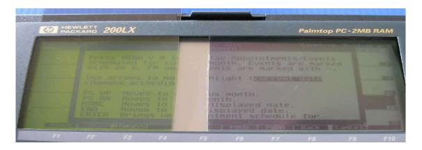
Now, in the photo above, the remnants of the 'transparent layer' on the HPLX screen have been scrapped off entirely. Overlaid on the left is a polarizer with the correct orientation (again, this same polarizer from my first attempt has the wrong orientation for the display but is now rotated 90 degrees to correct it). This is how a normal HPLX screen looked like without this curious 'transparent layer'. Notice the greenish sheen.
