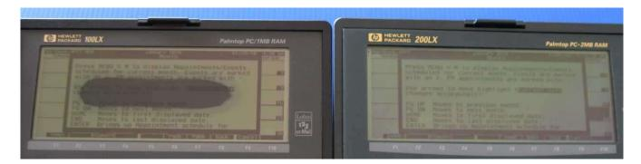
It's difficult to photograph the LCD screen contrasts clearly and accurately. The 200LX screen with the transplanted polarizer sheet is actually darker, greener, less clear and blemished with squashed bubbles but just about usable at the moment. This 200LX screen is not as clear and contrasty as the 100LX to begin with.
